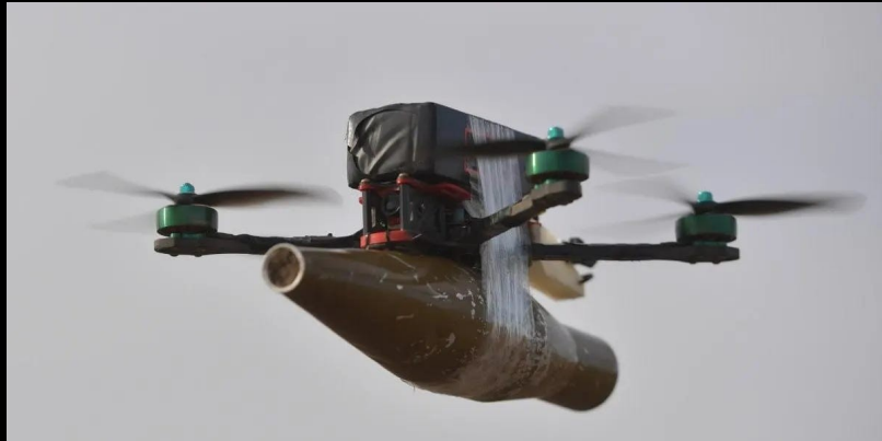
An FPV drone with an RPG-7 shell attached.
